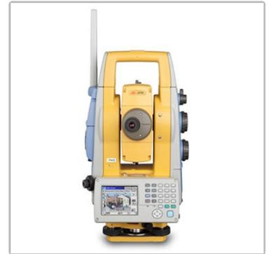
The IS's powerful functionality is controlled using Topcon's exclusive ImageMaster™ software that produces "photography with dimension", a revolutionary and cost-effective alternative to laser scanning.
